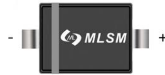
SOD-323 top view
