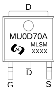
Marking and pin assignment
